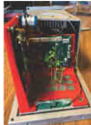
Plants growing inside the satellite vessel during an on-ground experiment
